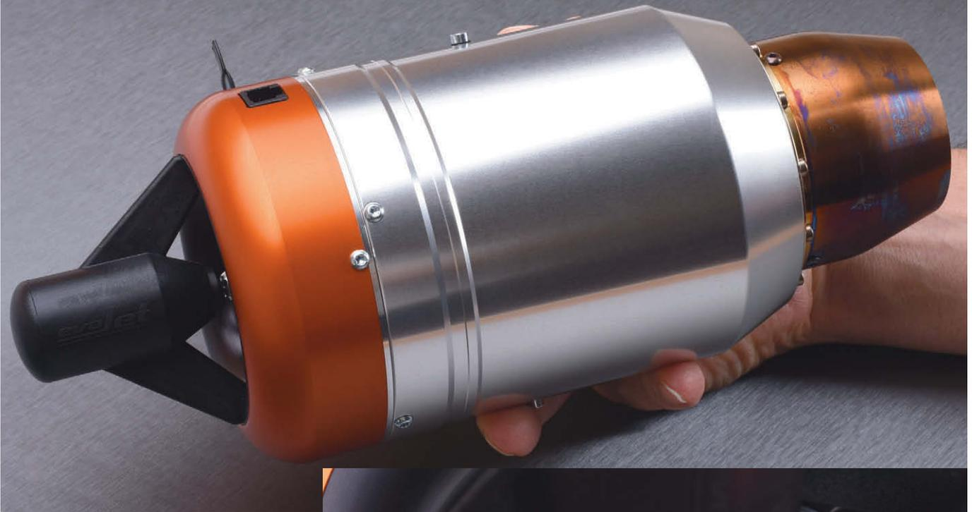
exceptionally clean, aided by the temperature sensor also being fitted internally, allowing a completely smooth and unbroken outer finish to the main casing, conventional clamp type mounts being used to secure the engine to the model, or in this case the test rig. All visible parts of the engine have been beautifully machined, and the impression of quality of design and manufacture is striking, the front cover being finished in an attractive orange colour.
