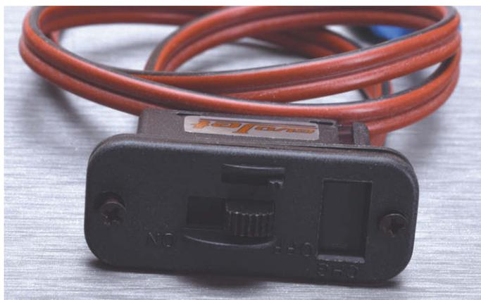
Unusually for a turbine, but very useful, a switch complete with charge socket is supplied with the engine.
