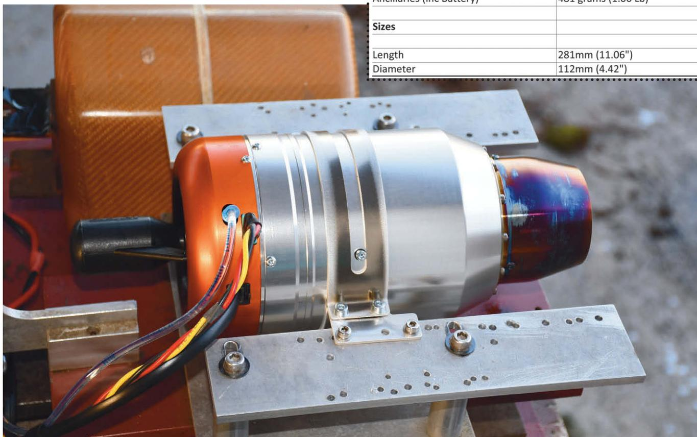
Ready for its first run, the B220neo sits on the test rig.
