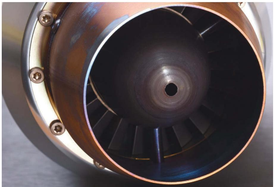
Tailcone and turbine wheel are equally nicely produced, note the unusual hole in the centre of the exhaust cone.
