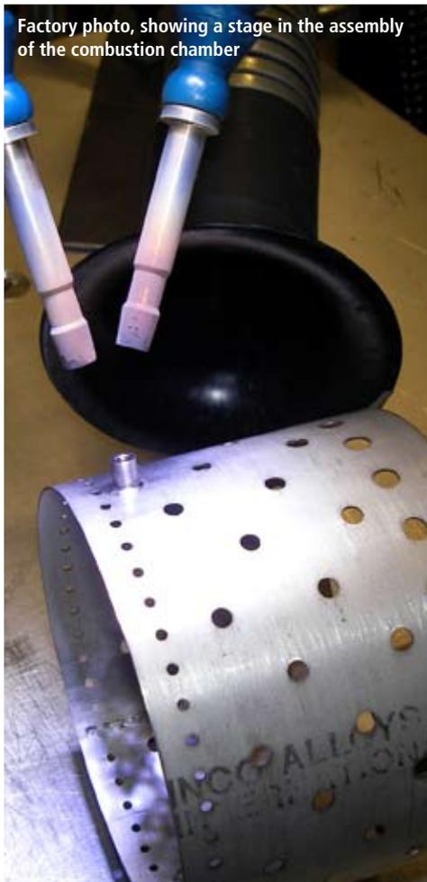
Factory photo, showing a stage in the assembly of the combustion chamber
