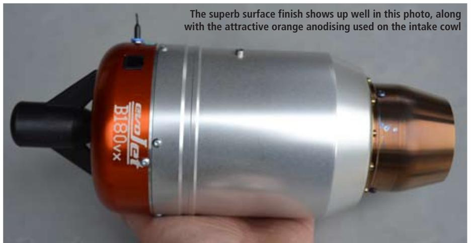
The superb surface finish shows up well in this photo, along with the attractive orange anodising used on the intake cowl
