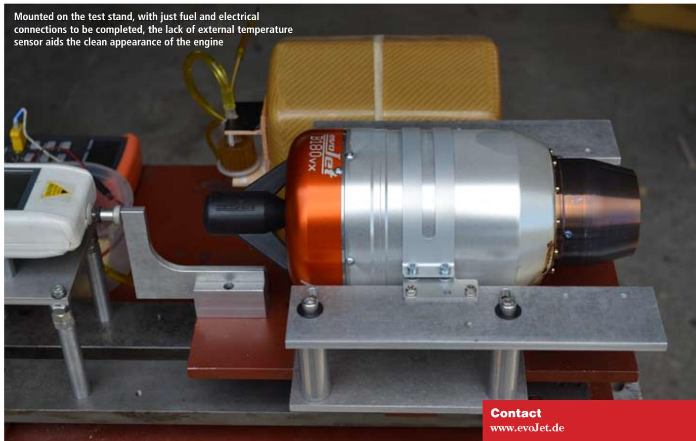
Mounted on the test stand, with just fuel and electrical connections to be completed, the lack of external temperature sensor aids the clean appearance of the engine
