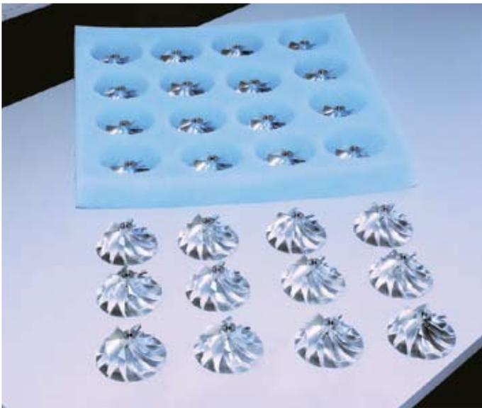
A batch of beautifully milled compressors ready to be assembled into engines
